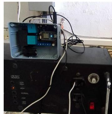
Fig. 6. IoTBPMU device installed at 127 VAC level.
