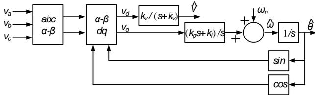
Fig. 1. SRF-PLL block diagram.
