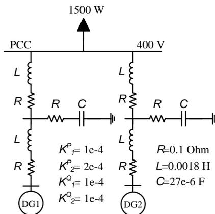
Fig. 11. Single line diagram of the three-phase test system.
