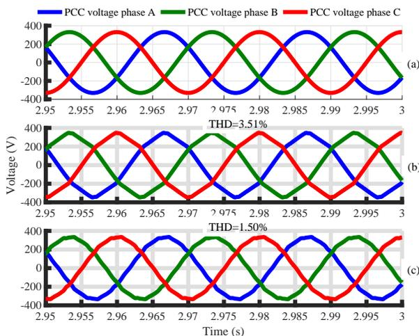
Fig. 17. Basic proportional-resonant control performance.
