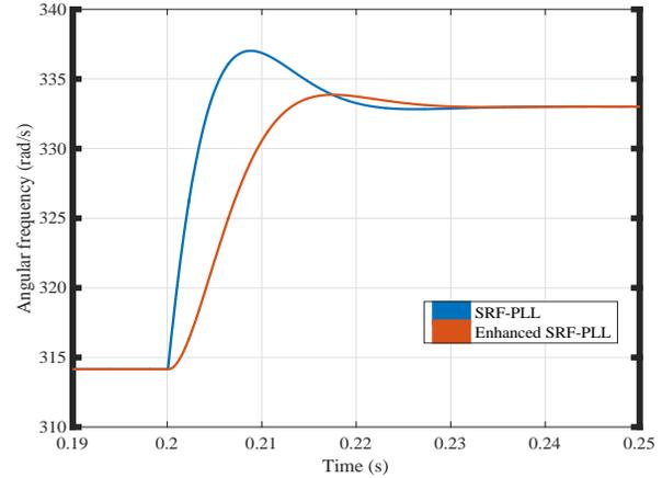
Fig. 8. Performance comparison between the conventional SRF-PLL and the Enhanced SRF-PLL in response to a 3 Hz frequency jump.
