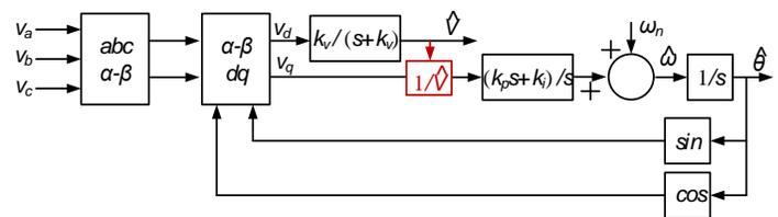
Fig. 3. SRF-PLL block diagram with normalization.
