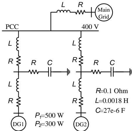
Fig. 14. Single line diagram of the three-phase test system for the connected case.
