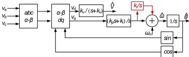
Fig. 5. SRF-PLL block diagram with an extra integrator.
