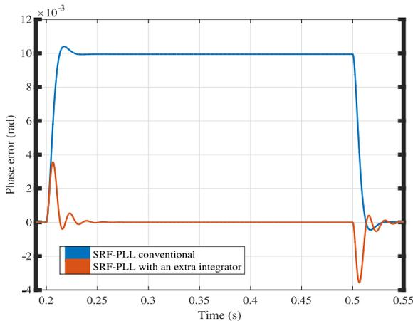
Fig. 6. SRF-PLL performance with and without the extra integrator, in response to a 30 Hz frequency ramp.
