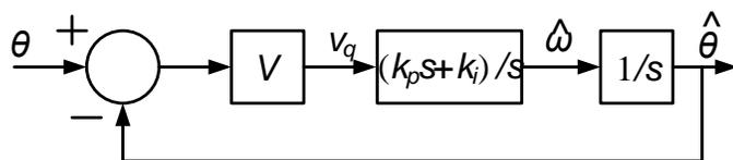
Fig. 2. SRF-PLL small-signal block diagram.
