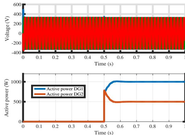
Fig. 12. PCC voltage and DG units injected active power during an energization and load connection.
