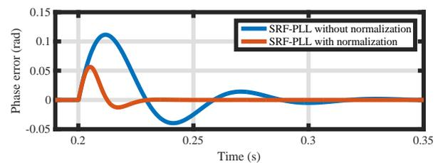
Fig. 4. SRF-PLL performance with and without amplitude normalization, in response to a voltage sag with 3 Hz frequency jump.
