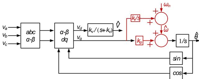
Fig. 7. Enhanced SRF-PLL block diagram.
